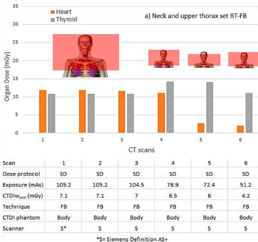
Fig. 2. Heart and thyroid doses of a RT-FB patient from the neck and upper thorax set, that received 8 CT scans. The scan range is illustrated on top of the corresponding CTs for the patient. The image of the scanning regions was taken by the output files of VirtualDose. Relevant data about imaging protocol, such as exposure and CTDI_{w_aver} , from each CT is represented below the plot. The kVp value was 120 for all the scans.
