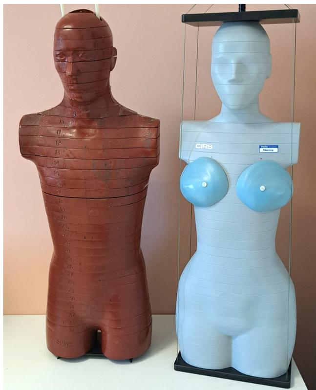
**FIGURE 3** The male (left) and female (right) anthropomorphic phantoms used for physical absorbed dose measurements using thermoluminescent detectors.
